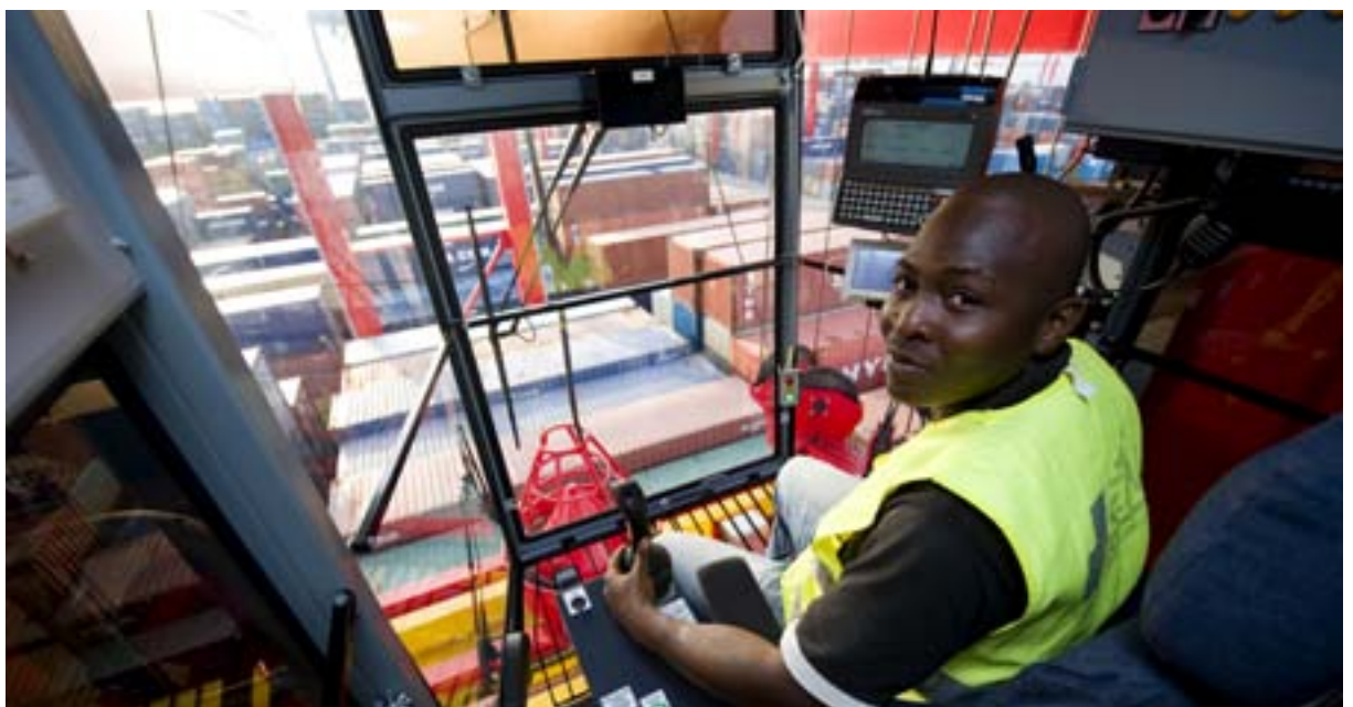
■ Crane Operator Julien Tahno Say moves cranes from the cabin of a Konecranes RTG crane.
