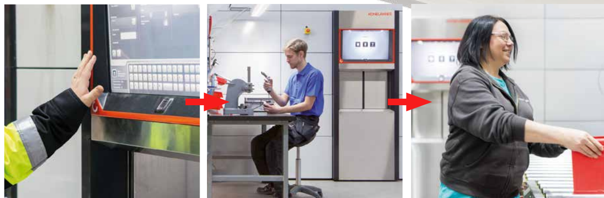
Incoming items are received directly by Agilon and data transferred to the enterprise resource planning system.
