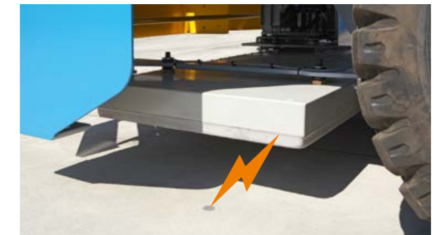
The transponder system, familiar from the Konecranes Gottwald AGV, is based on passive transponders in the terminal ground and surface antennas on the equipment side
