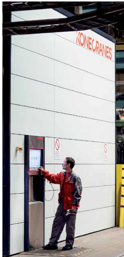
Hydraulics fitter Tommi Kemppinen uses the Agilon system at the user access point.
